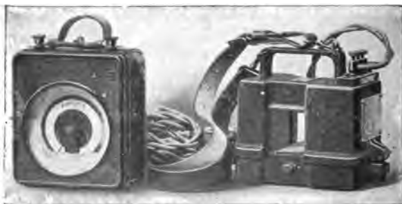
FIG. 183a. Portable series or current transformer. Westinghouse Electric and Mfg. Co.
